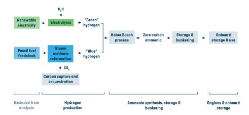
**Figure 3:** Zero carbon ammonia production chain
